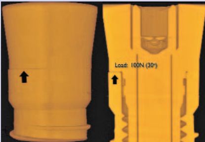
FIGURE 7 —These \mu CT images show that micro-gaps at the implant-abutment interface can engender adverse effects. These including screw loosening, abutment rotation, abutment fracture and peri-implantitis. Interface gapping/pumping is reported to be associated with progressively negative biological changes and the continuous mobility between components imperils wound healing around the implant. Tissue response induced by inflammatory vectors can be as aesthetically disastrous as that induced by impingement on the biologic width in the natural tooth scenario.
